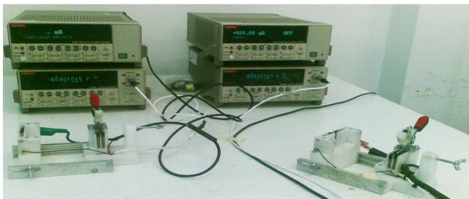
The system for measuring the contact resistance between terminals and electrical cables (Cable Wire **Terminal Connector Contact Resistance Meter**), **TermResMeter**, is designed for automatic and semi-automatic measurements of contact resistance between different sized and shaped terminals and single core, multi core, tape, bar or any other type of electrical cables. This system enables contact resistance measurements in any point of contact.
